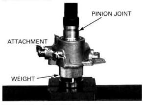
Install the snap ring into the pinion joint groove securely with the chamfered edge facing the bearing.
