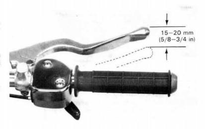
Adjust free play by turning the adjusting nut.
